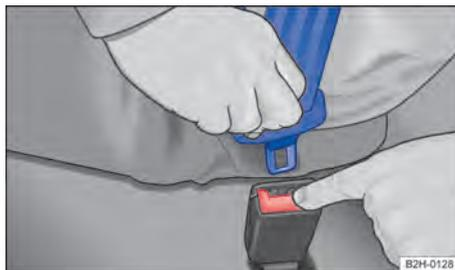
Fig. 36 Removing the latch plate from the buckle
