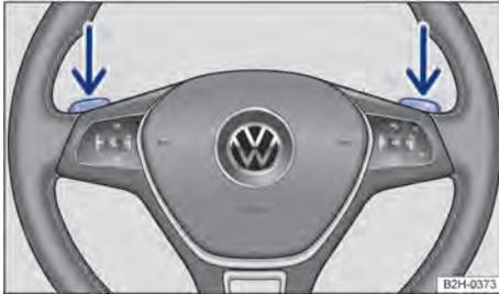
**Fig. 105** Steering wheel with Tiptronic gear shift paddles.
