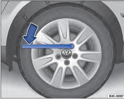
**Fig. 202** Changing a wheel: loosening the wheel bolts.
