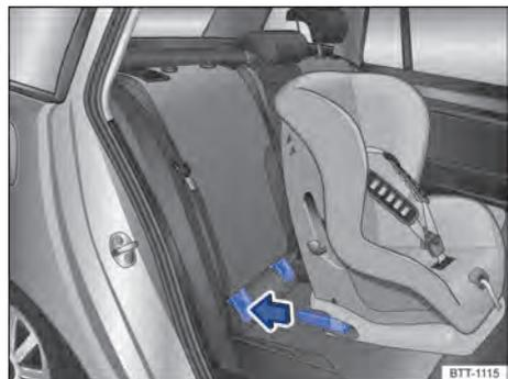
**Fig. 53** Schematic representation: installing the ISOFIX child seat with the support arms.
