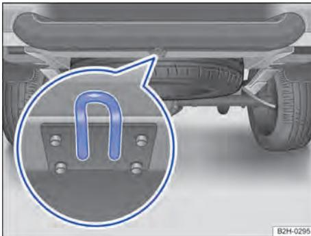
**Fig. 176** Below the bumper: towing eye on vehicles without factory towing device.
