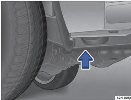
Fig. 214 From the side: The front jacking point.
