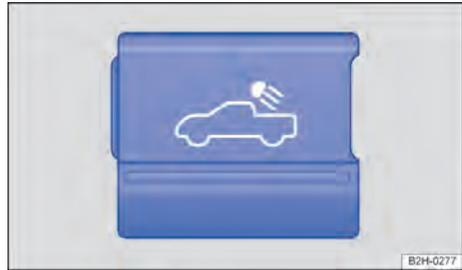
**Fig. 87** In the centre console: Button for loadbed lighting.
