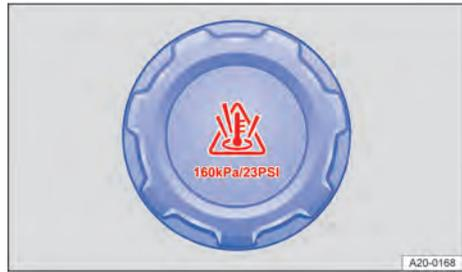
Fig. 189 In the engine compartment: coolant expansion tank cap
