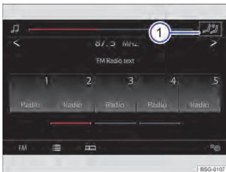
**Fig. 128** Screen display in the centre console: Function button for opening the Voice Enhancer.
