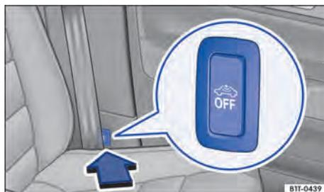
**Fig. 60** Next to the driver seat: button for switching off the interior monitoring and the anti-tow alarm.
