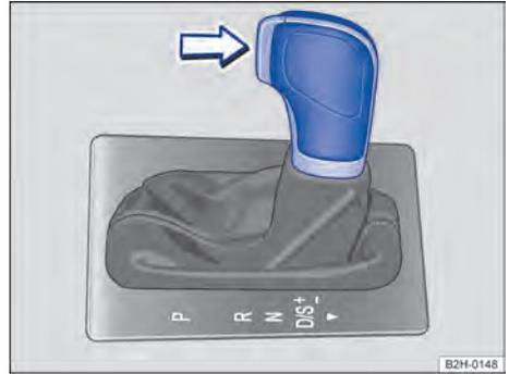
**Fig. 103** Left hand drive: automatic gearbox selector lever with interlock button (arrow). On right-hand drive vehicles, the arrangement of the elements is mirrored.
