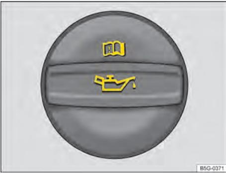
**Fig. 188** In the engine compartment: engine oil filler opening cap (illustration).
