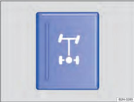
**Fig. 112** In the centre console: button for the differential lock (illustration).
