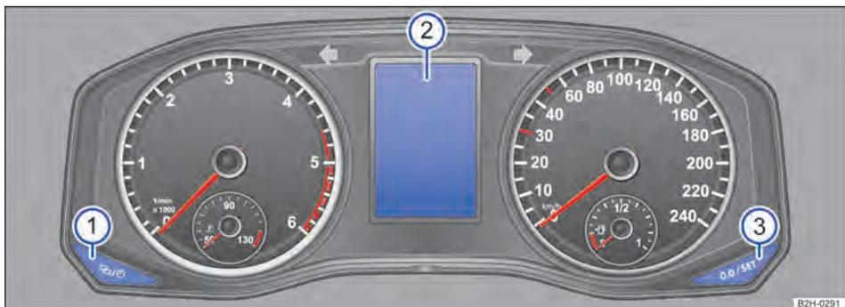
**Fig. 195** Buttons in instrument cluster in the dash panel.
