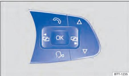
Fig. 11 On the multifunction steering wheel: Buttons for operating the menus in the instrument cluster.
