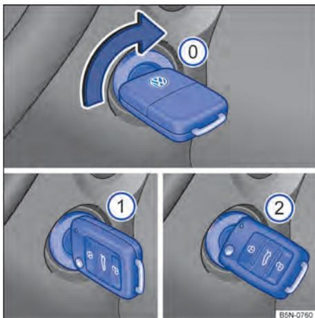
**Fig. 101** Next to the steering wheel on the right: Positions of the vehicle key in the ignition lock
