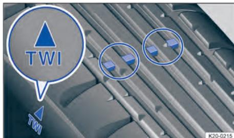
Fig. 199 Tyre tread: tread wear indicators.
