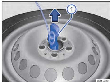
Fig. 208 Spare wheel or temporary spare wheel: Releasing the wheel holder.
