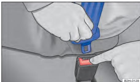
**Fig. 34** Removing the latch plate from the buckle
