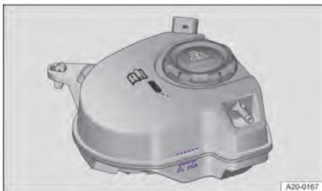
**Fig. 190** In the engine compartment: mark on the coolant expansion tank (illustration).
