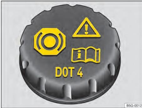
**Fig. 192** In the engine compartment: brake fluid reservoir cap.
