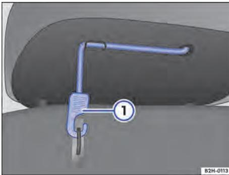
**Fig. 70** Under the rear bench seat: Retaining strap on the seat cushion.
