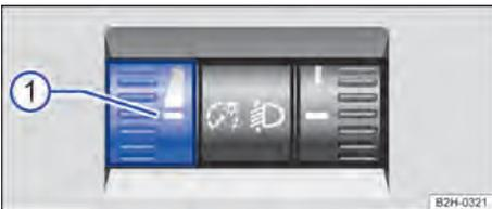
**Fig. 86** Beside the steering wheel: Controls for instrument and switch lighting.
