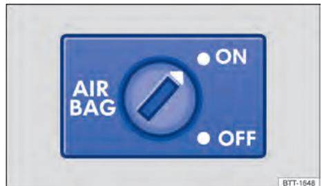
**Fig. 43** On the face end on the front passenger side: key-operated switch for switching the front passenger front airbag on and off.
