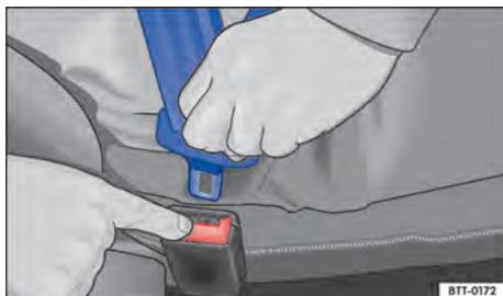
**Fig. 32** Removing the latch plate from the buckle
