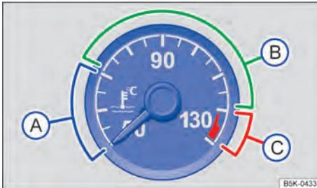
**Fig. 14** Coolant temperature display in the analogue instrument cluster (schematic diagram).
