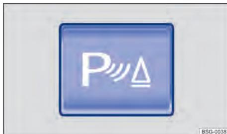
**Fig. 119** In the centre console: button for switching the Park Distance Control on or off (with some equipment levels).
