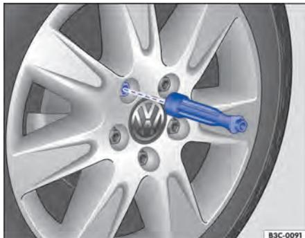
**Fig. 219** Changing a wheel: removing the wheel bolts with the screwdriver handle.
