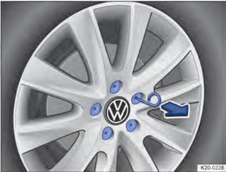
Fig. 201 Removing the wheel bolt caps.
