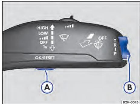
Fig. 12 On the wiper lever: Buttons for operating the menu.
