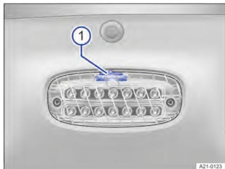
**Fig. 88** Above the tailboard: Switch for hardtop lighting.
