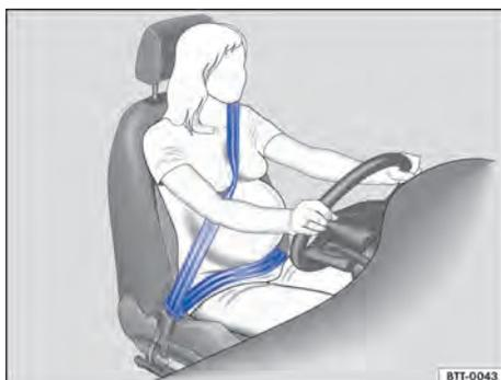
Fig. 38 Correct seat belt routing during pregnancy
