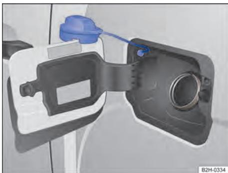
**Fig. 150** On the left-hand side of the vehicle: tank flap with open tank cap.
