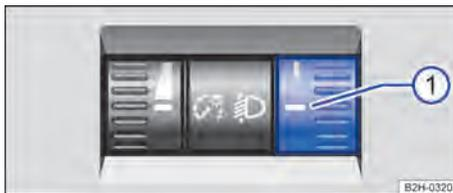
**Fig. 85** Beside the steering wheel: Headlight range control ①.
