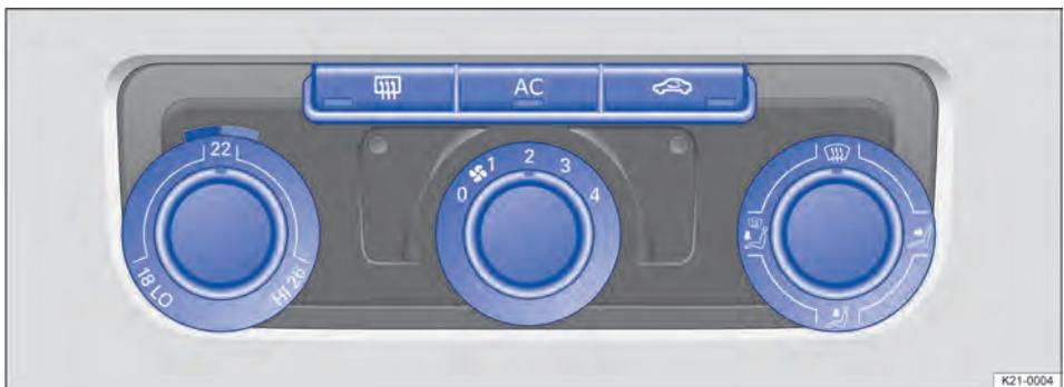
Fig. 96 In the dash panel: Air conditioning system controls.
