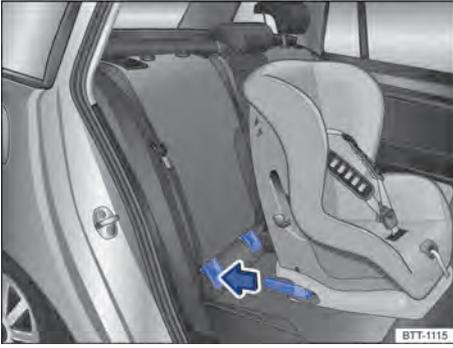
**Fig. 51** Schematic representation: installing the ISOFIX child seat with the support arms.
