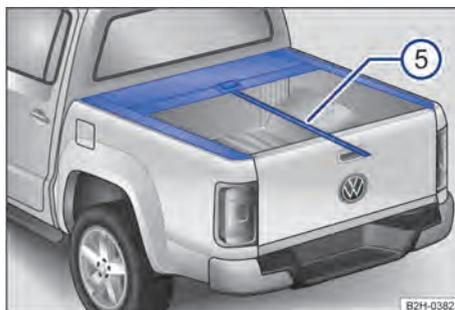
Fig. 64 Cargo compartment sea roof: traction strap
