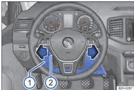
Fig. 170 On the driver side, left-hand drive vehicle: Fuse box behind the dash panel trim.
