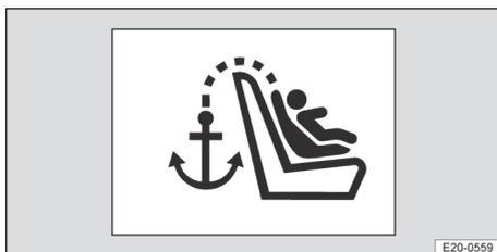
Fig. 54 Illustration: label showing the top tether attachment point.
