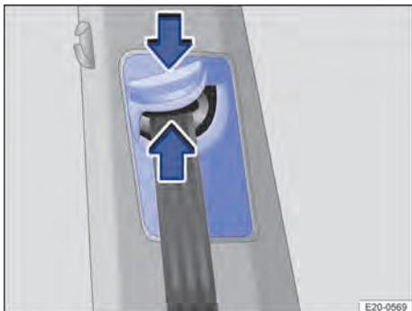
**Fig. 39** Next to the front seats: seat belt height adjuster.
