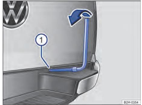
**Fig. 211** Place the spare wheel on the winch.
