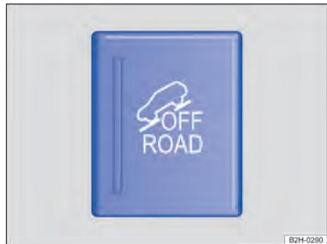
**Fig. 108** In the centre console: Button for switching the offroad function on and off manually.
