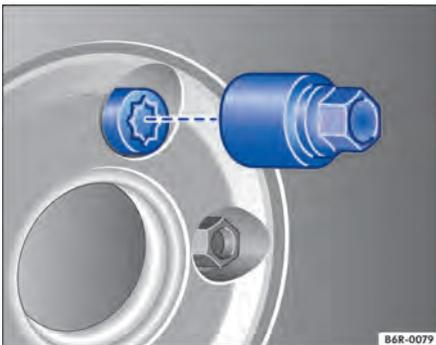
**Fig. 203** Changing a wheel: Anti-theft bolt and adapter.
