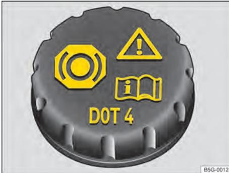
**Fig. 195** On the engine compartment: brake fluid reservoir cap.
