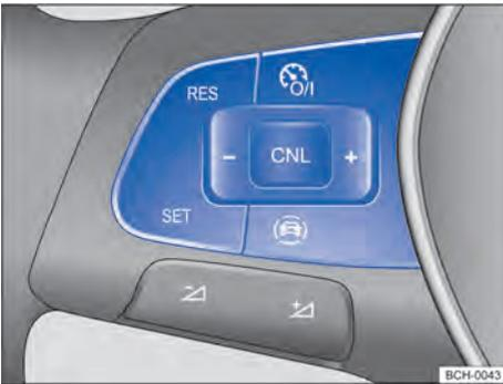
**Fig. 96** Left side of the multifunction steering wheel (version 1): GRA operating buttons.
