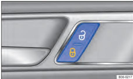
**Fig. 51** On the driver door: central locking button.
