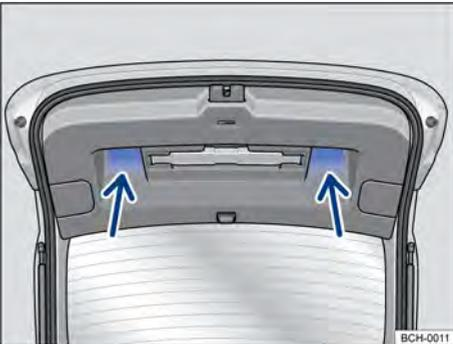
Fig. 57 Open boot lid: recesses (arrows) to pull and close.
