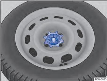
Fig. 202 On the luggage compartment: spare wheel fastening handwheel.
