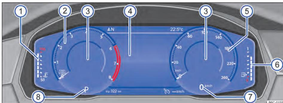
Fig. 9 Active Info Display (version 1) on the dash panel.
