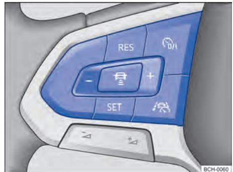
Fig. 104 Left side of the multifunction steering wheel: ACC operating (variant 2) buttons.
