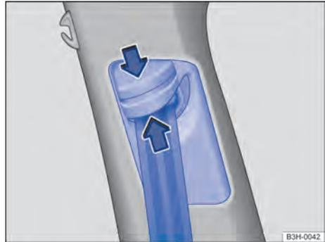
**Fig. 31** Next to the front seats: seat belt height adjuster.
