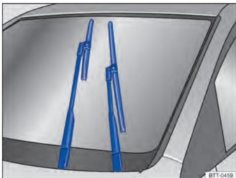
Fig. 173 Window wipers in service position.
