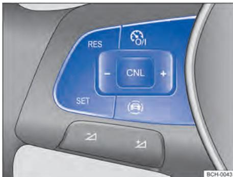
Fig. 98 Left side of the multifunction steering wheel (version 1): speed limiter operating buttons.
