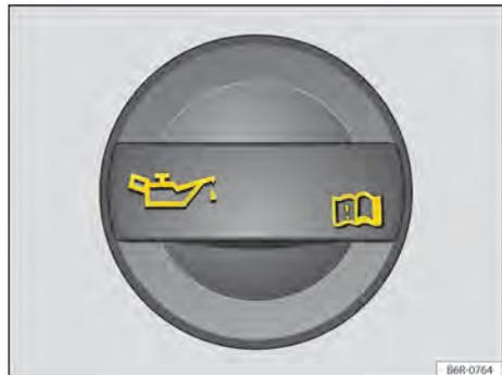
Fig. 192 On the engine compartment: engine oil opening lid.
