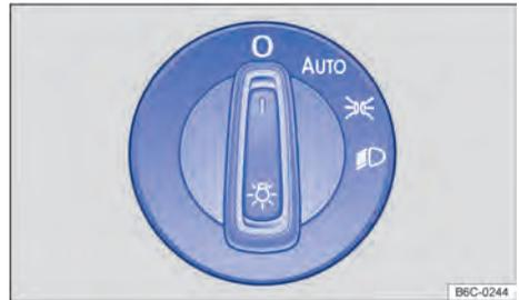
**Fig. 69** Next to the steering wheel: light switch (one variant).
