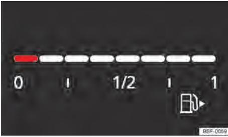
**Fig. 12** On the digital instrument cluster: fuel gauge (version 2).
