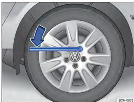
Fig. 204 Changing the wheel: loosen wheel bolts.
