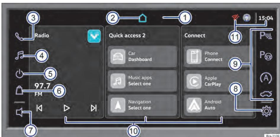
Fig. 153 Overview of controls (variant 1).
