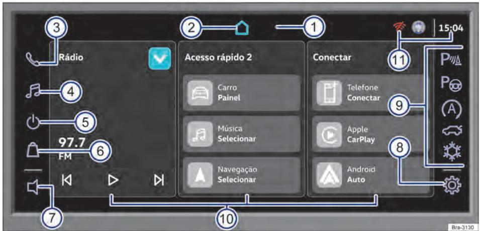
**Fig. 154** Overview of controls (variant 2)
