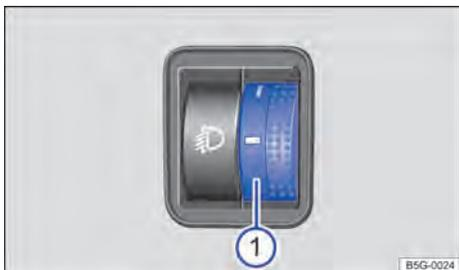
**Fig. 71** Next to the steering wheel: control of the headlight range ①
