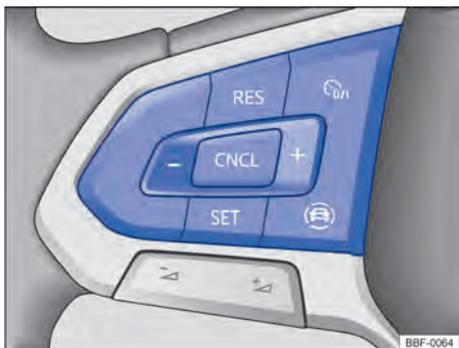
**Fig. 99** Left side of the multifunction steering wheel (version 2): speed limiter operating buttons.
