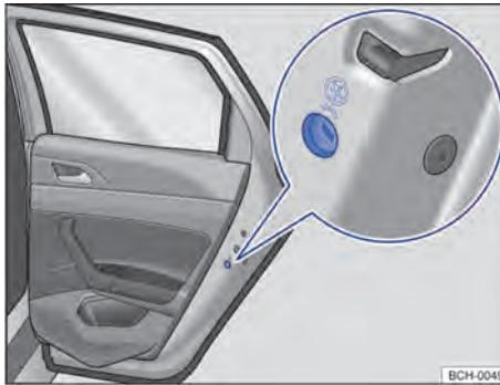
**Fig. 44** On the rear door (right-hand side): childproof lock.
