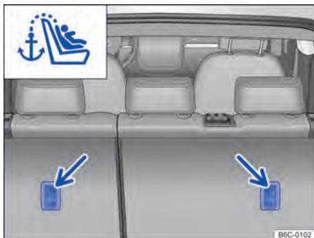
Fig. 42 retention eyes for the top tether on the back side of the rear seat.
