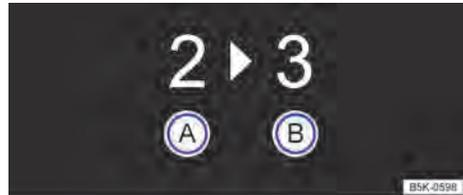
**Fig. 84** On the instrument cluster: gear change indicator.
