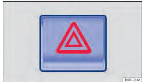
**Fig. 45** On the upper portion of the centre console: warning lamp switch.
