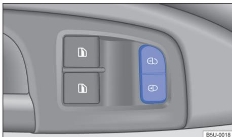
Fig. 42 On the driver door: central locking button.
