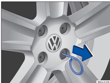
**Fig. 168** Removing the wheel bolt caps.
