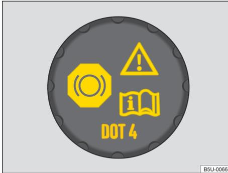
**Fig. 158** On the engine compartment: brake fluid reservoir cap.
