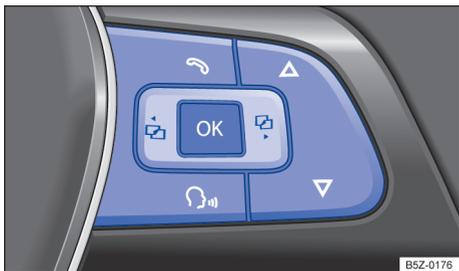
**Fig. 18** Right-hand side of the multifunction steering wheel: instrument cluster menu control buttons.
