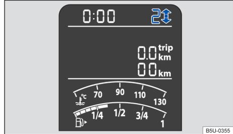
Fig. 79 On the instrument cluster: gearshift indicator (variable 1).
