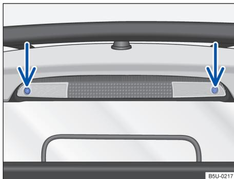
Fig. 141 On the bed: remove the elevated brake light.
