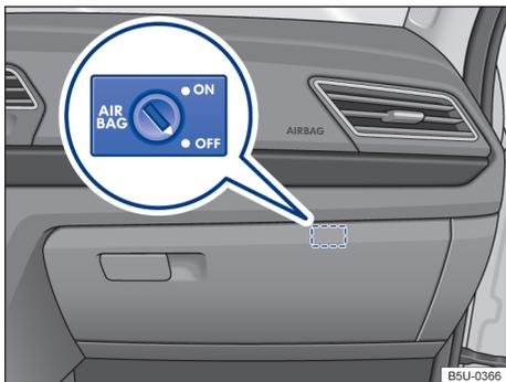
**Fig. 35** On the stowage compartment: switch deactivated by the key to switch the passenger front airbag on and off.
