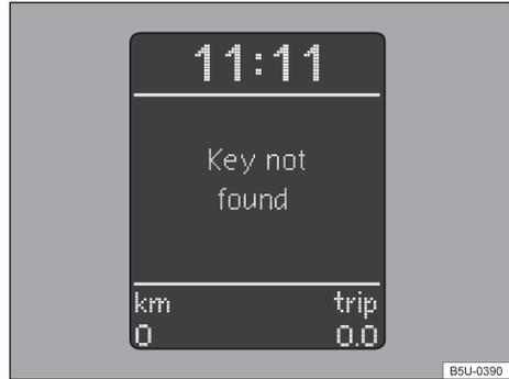
**Fig. 83** On the instrument cluster: display indicating the activated immobilizer - vehicles with Volkswagen Information System.
