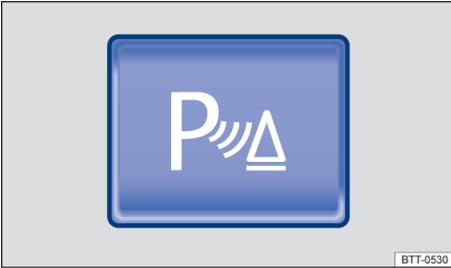
**Fig. 89** On the upper part of the centre console: parking distance control on/off button (Park Pilot).
