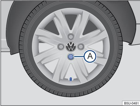
Fig. 169 Removing the wheel covers.
