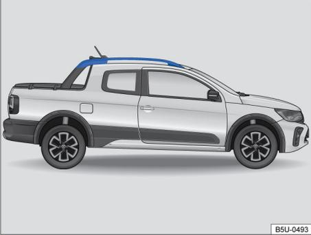
**Fig. 123** Roof rack longitudinal supports (both sides).
