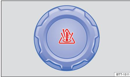
**Fig. 174** On the engine compartment: engine coolant expansion tank cover.
