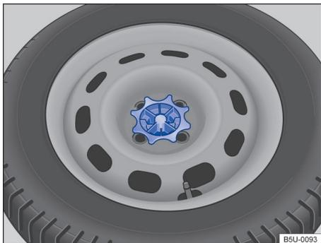
**Fig. 182** On the luggage compartment: spare wheel fastening handwheel.
