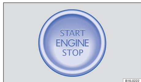
**Fig. 91** On the lower part of the centre console: engine start button.
