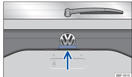
Fig. 56 On the boot lid: button to open the boot lid.
