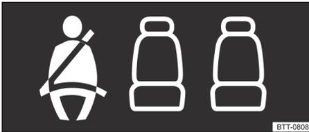
Fig. 21 Seat belt status indicator for rear seats in the instrument cluster display.
