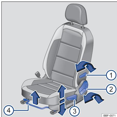
Fig. 62 On the front seat: controls.
