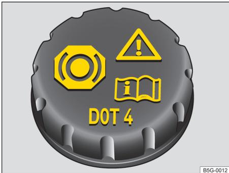
**Fig. 175** On the engine compartment: brake fluid reservoir cap.
