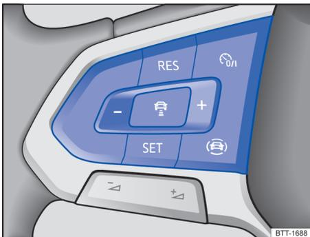
Fig. 110 Left side of the multifunction steering wheel: ACC operating buttons.
