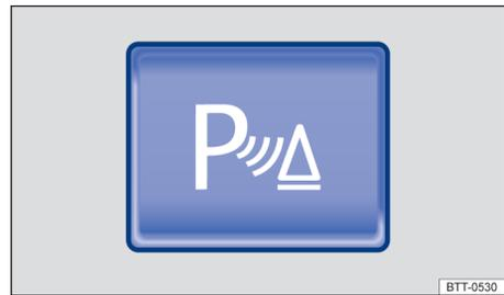
**Fig. 115** On the centre console: manual park distance control on/off button.
