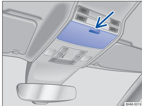
**Fig. 128** In the roof console: glasses compartment.
