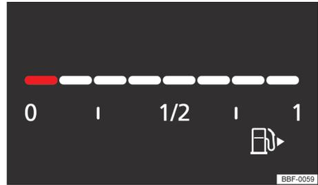
Fig. 12 On the digital instrument cluster: fuel gauge (version 2).
