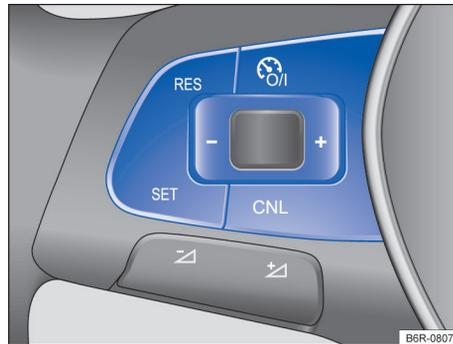
Fig. 103 Left side of the multifunction steering wheel (version 1): GRA operating buttons.
